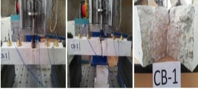
Fig. 4 Damage development of the specimen
