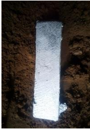
Plate 5: An Aluminium Cast Products using Nasarawu Natural Sand at 6% Moisture Content
