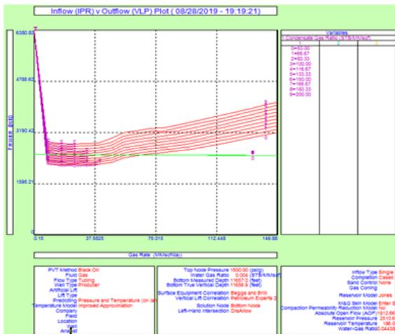
Fig 6: Condensate- Gas Ratio VLP (or TPC) Sensitivity
