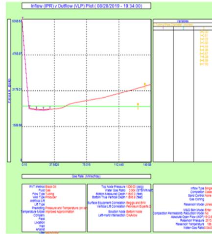
Fig 7: Tubing Size - Tubing Vertical Lift Performance Sensitivity Analysis
