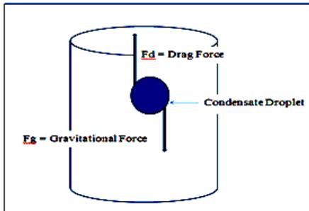
Fig 1: Turner's Liquid Droplet Model
