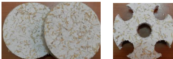
Figure 2. Acoustic cell specimens before and given a Helmholtz resonator
