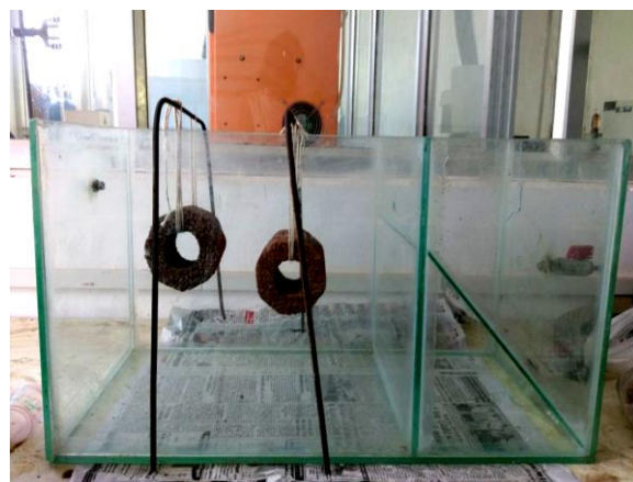
Fig no.5.1: Arrangement of Eco Bio-blocks in the reactor
