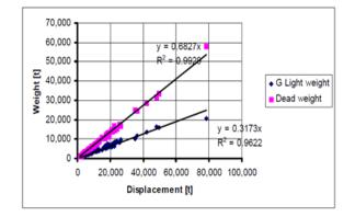
Figure 2 Plot of Weight against Displacement in Tonnes for Light and Dead Weights [7]
