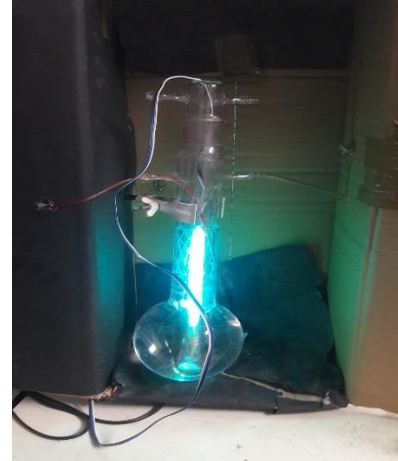
Fig:1 schematic diagram of UV/H 2 O 2 reactor Fig:2 Laboratory experimental setup Fig:3 Reactor under UV
