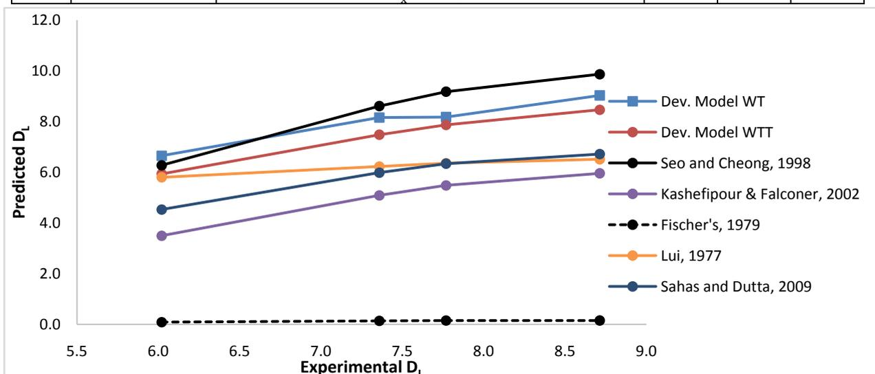
**Fig. 4: Predicted Against Experimental Dispersion Coefficient for Different models**
