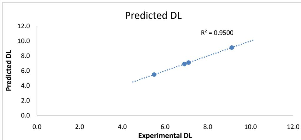
**fig. 2: Predicted Dispersion Against Experimental Dispersion Values (model calibration)**
