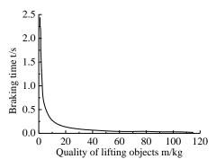
Fig.6 Braking System Braking Time
