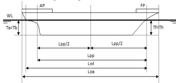
**Fig.1: Longitudinal Shape of the Vessel**
