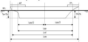
Fig.1: Longitudinal Shape of the Vessel
