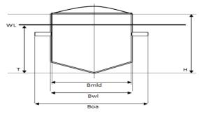
Fig.2: Cross-sectional Shape of the Vessel
