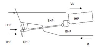
Fig.3: Propulsion System of the Vessel
