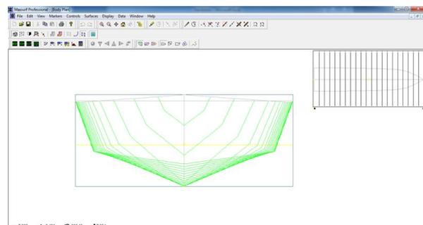
Fig.7: The Body Display Plan of the Indonesian Navy Vessel
