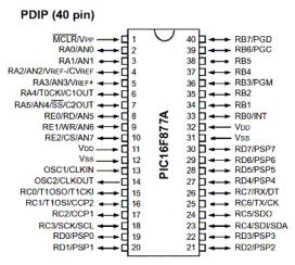
Fig. 6: Schematic of the 40-pin [6] PIC16F877A
