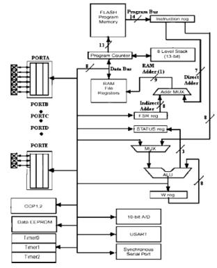
Fig. 7: Internal Diagram of PIC16F877A
