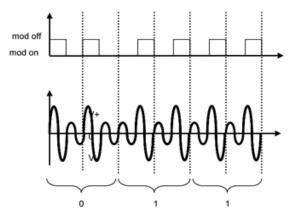
Fig. 4: Wave Diagram of the Logic 1's and 0's [4]
