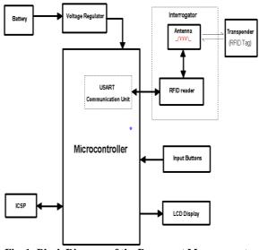
Fig. 1: Block Diagram of the Document Management RFID System
