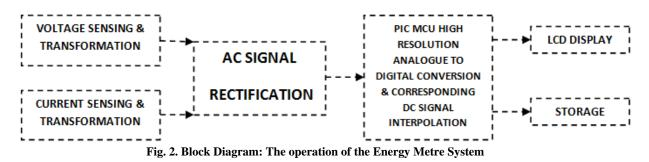
The sections below shed more light on the various stages involved in the metering process.
