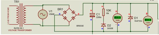
Fig. 3: Schematic of the Voltage Transformational System
