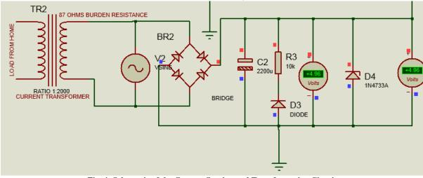
Fig. 4: Schematic of the Current Sensing and Transformation Circuit
