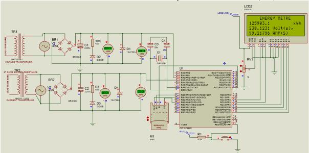
Fig. 1. Schematic of the Digitalized Energy Metre
