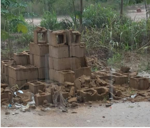
Fig. 1 Deteriorating concrete hollow blocks of 450*225*225 mm size
