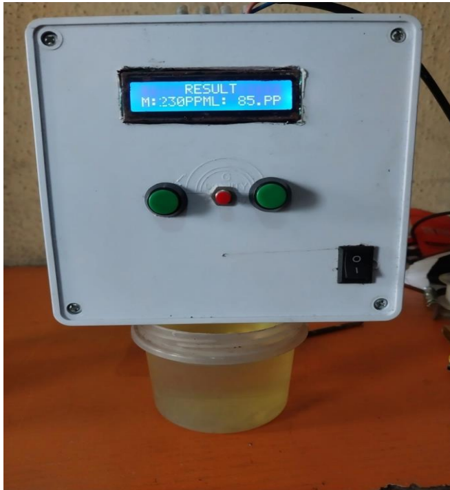
Fig. 4 Fuel adulteration detection system
