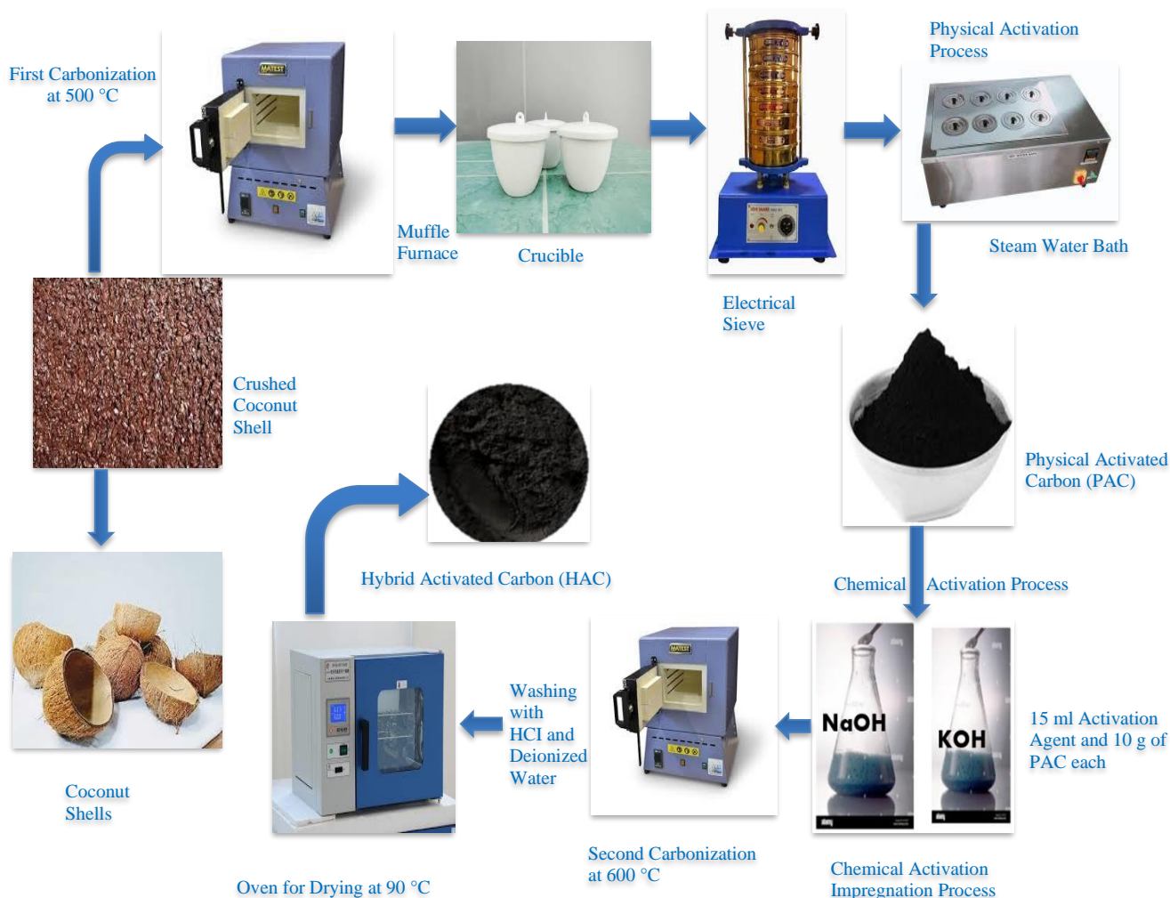
Fig. 2 Synthesis of Bio-based activated carbon electrode material
