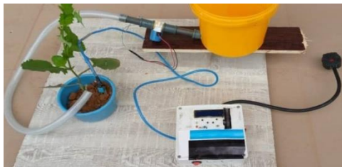
Fig. 10 Finished time-based automated irrigation system
