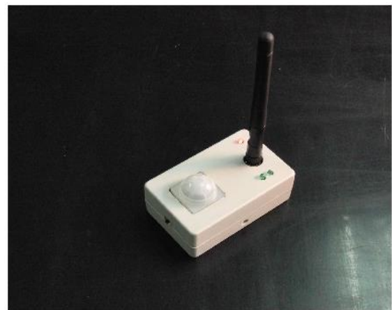
Figure5. A prototype of the PIR Sensor node
