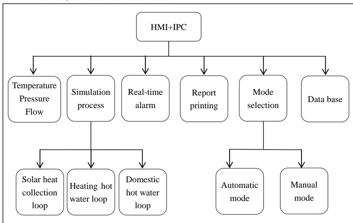
**Figure.2 Structure Diagram of Monitoring System**
