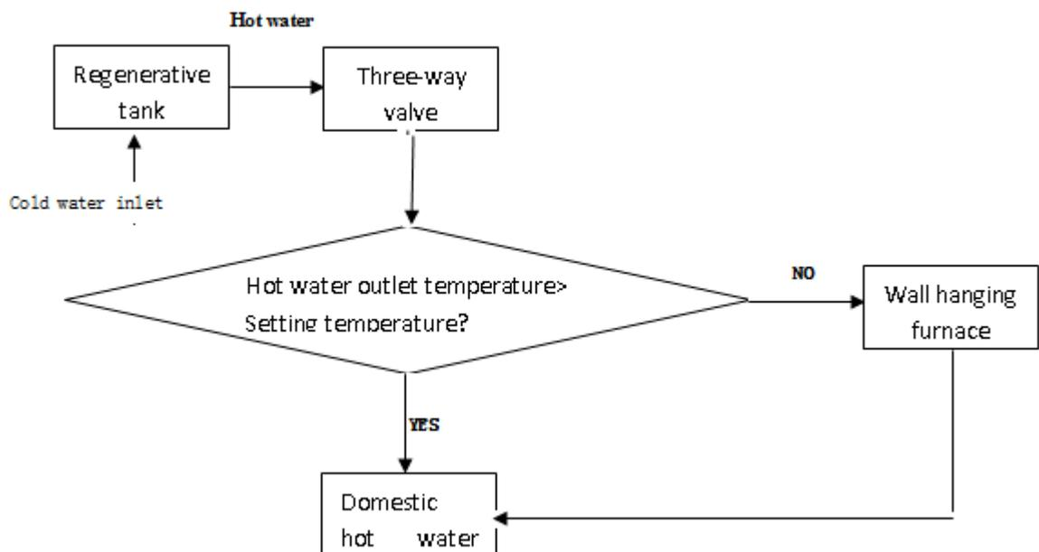
**Figure.1 Life Hot Water Loop Flow Chart**
