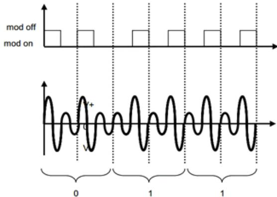
Fig. 4: Wave Diagram of the Logic 1's and 0's [4]
