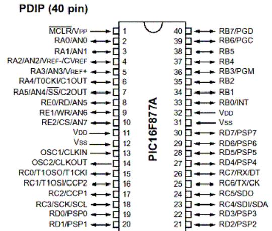
Fig. 6: Schematic of the 40-pin [6] PIC16F877A
