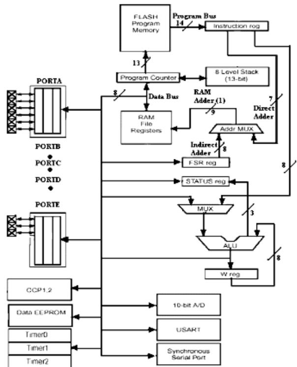
Fig. 7: Internal Diagram of PIC16F877A
