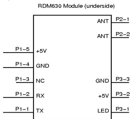
Fig 5: Schematic of the Reader Module [5]
