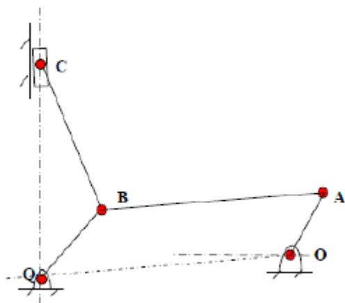
Fig.1 The 6 bar-1 slider mechanism [10].
