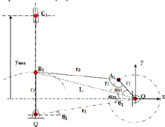
Fig.2 The mechanism in its first limiting position [10].
