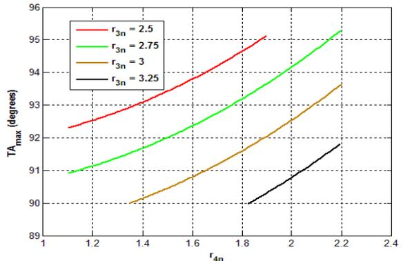
Fig.7 Mechanism maximum transmission angle.
