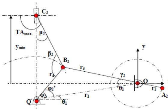
Fig.3 The mechanism with slider in its lower limiting position.
