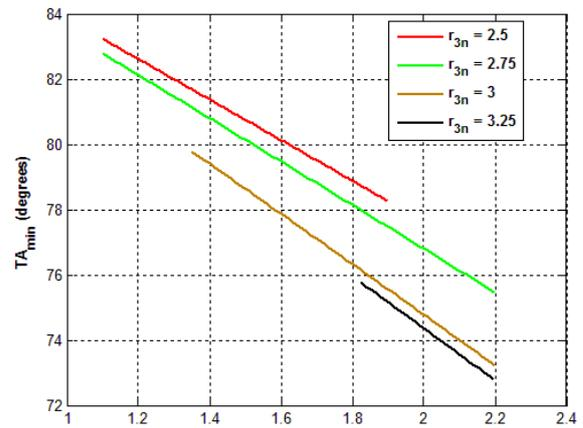
Fig.6 Mechanism minimum transmission angle.
