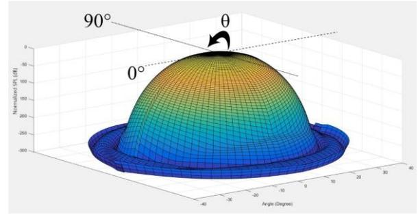
**Fig. 5. Directivity for the circular microphone array with 57 microphones for  $\theta = 60^\circ$  using delay-and-sum beam-forming and optimization method. (3D)**
