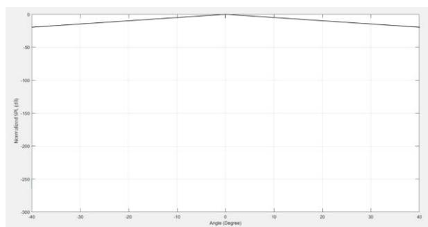
Fig. 1. Directivity for the microphone array with 8 microphones for  $\theta = 30^\circ$  using the delay-and-sum beam-forming method.
