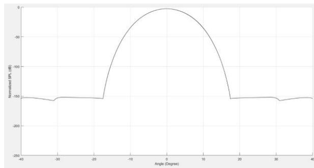
Fig. 2. Directivity for the circular microphone array with 57 microphones for  $\theta = 30^\circ$  using delay-and-sum beam-forming and optimization method.
