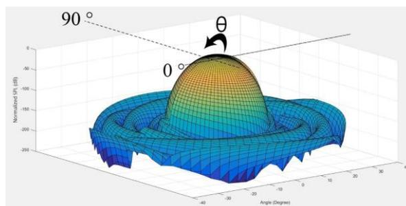
Fig. 3. Directivity for the circular microphone array with 57 microphones for  $\theta = 30^\circ$  using delay-and-sum beam-forming and optimization method. (3D)
