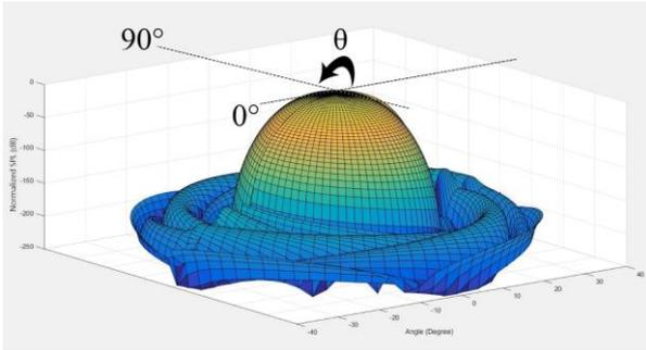
**Fig. 4. Directivity for the circular microphone array with 57 microphones for  $\theta = 40^\circ$  using delay-and-sum beam-forming and optimization method. (3D)**
