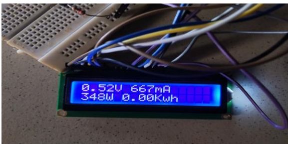
Figure 12: Voltage, Current and Energy Readings at no Load
