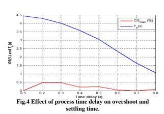
The settling time decreases nonlinearly as the time delay increases. The maximum percentage overshoot changes between zero and 0.47 % during the time delay range between 0.1 and 0.8 s.
