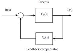
Fig.2 Closed-loop control system.
