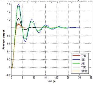
Fig.2 Control system time response for a 0.2 s time delayed double integrating process.
