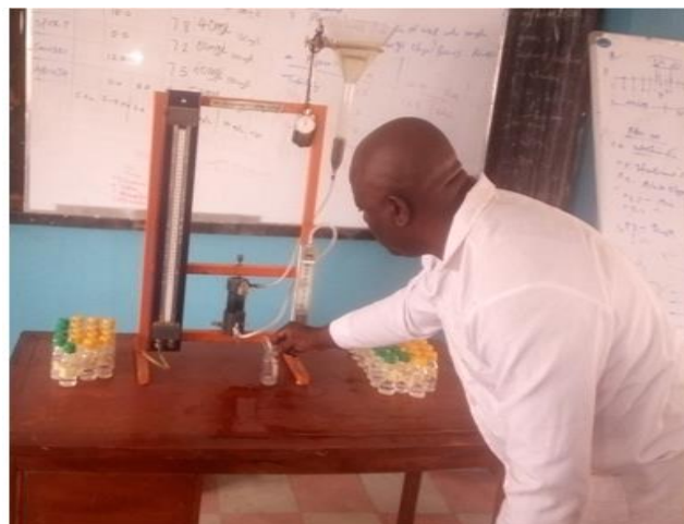
Plate 4. Experimental set-up of column adsorption for the study
