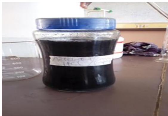
Plate 3. Impregnation of carbonized OGL in NaOH – Activation process
