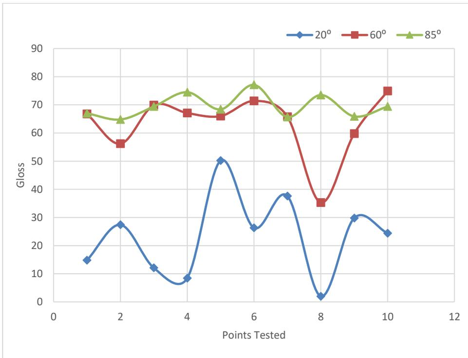
Fig. 3: Gloss of the paint finish by M.A Motors (Sample B)
