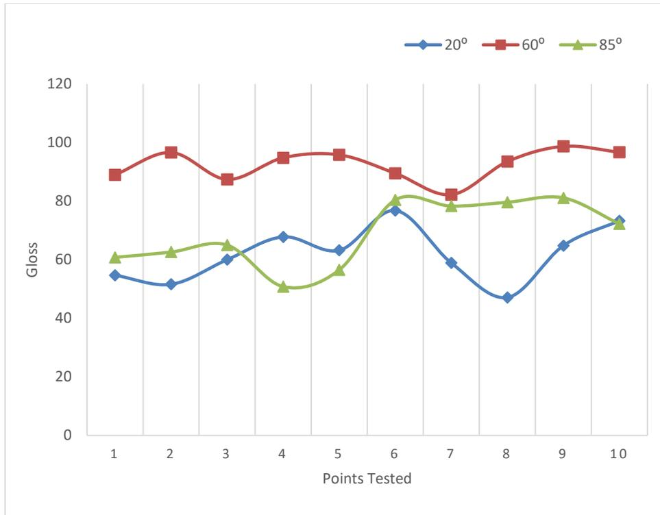
Fig. 4: Gloss of the paint finish by Alsarafa Body Painters (Sample C)
