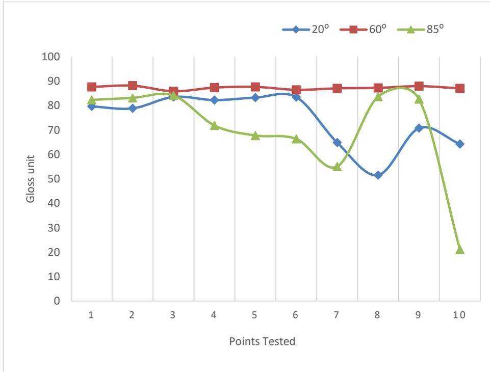
Fig. 2: Gloss of the paint finish by PAN (Sample A)
