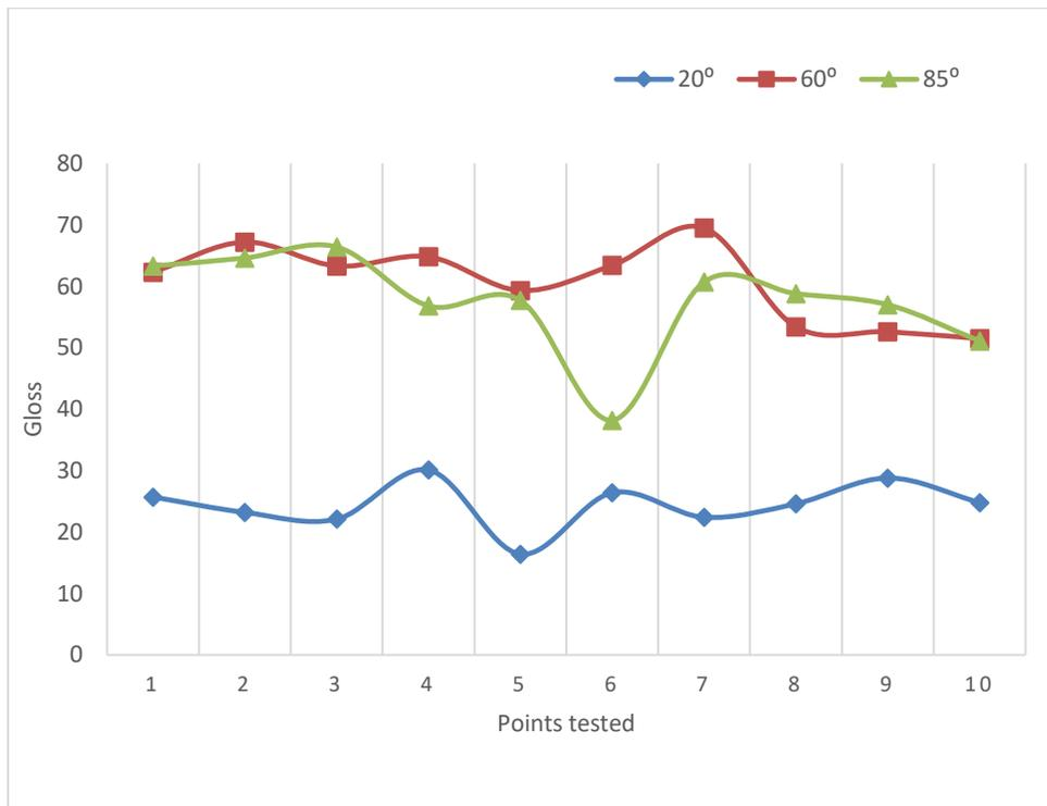
Fig. 5: Gloss of the paint finish by I.B.K Motors (Sample D)
