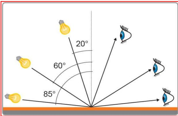
Fig. 1: Angles of the gloss measurements [6]
