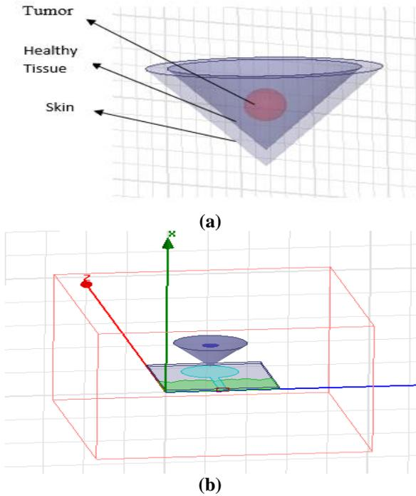
Figure 4: (a) Breast model (b) Breast model with antenna
