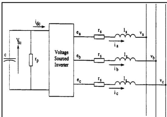
**Fig.1: Equivalent Circuit Of STATCOM**
