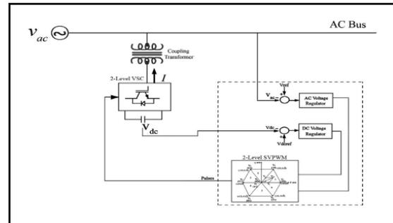
**Fig.7: Two-Level Svpwm Controlled Statcom**
