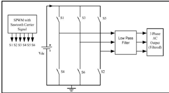
**Fig.5: Block Diagram Of SPWM Based Three Phase Inverter Using Triggering Circuit And Low Pass Filter**
