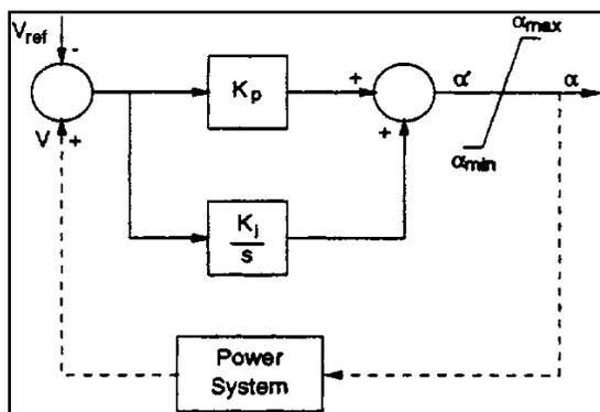
**Fig.2: Block Diagram Of PI Control Scheme**
