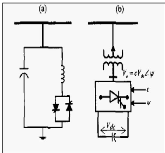
Fig.3: Schematic Diagram Of (A) SVC And (B) STATCOM
