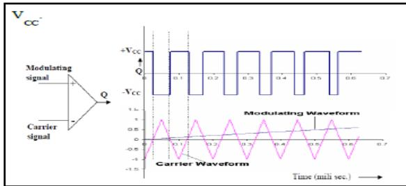
**Fig. 6: Waveforms For Comparison Of Modulating And Carrier Signals**
