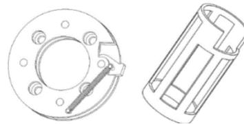
Fig.1 : brake disc Fig.2 fixed stop
