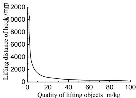
**Fig.7 Lifting Distance of Hook**
