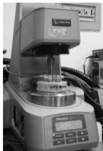
(a) Rheometer Physica MCR301
