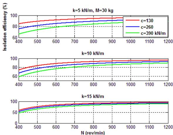
Fig.7 Isolation efficiency for  $M=30$  kg.
