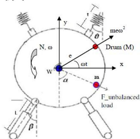
Fig.1 Horizontal washing machine physical model [10], [11].
