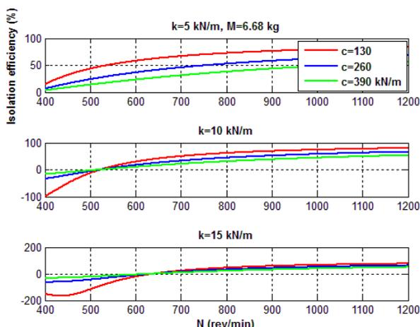
Fig.5 Isolation efficiency for  $M=6.68$  kg.
