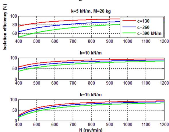
Fig.6 Isolation efficiency for  $M=20$  kg.
