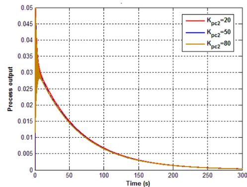
**Fig.5 Effect of the controller gain  $K_{pc2}$  on the disturbance time response.**
