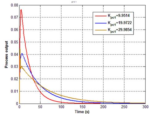
**Fig.3 Effect of the controller gain  $K_{pc1}$  on the disturbance time response.**
