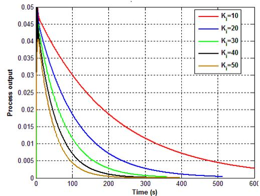
**Fig.4 Effect of the controller gain  $K_i$  on the disturbance time response.**
